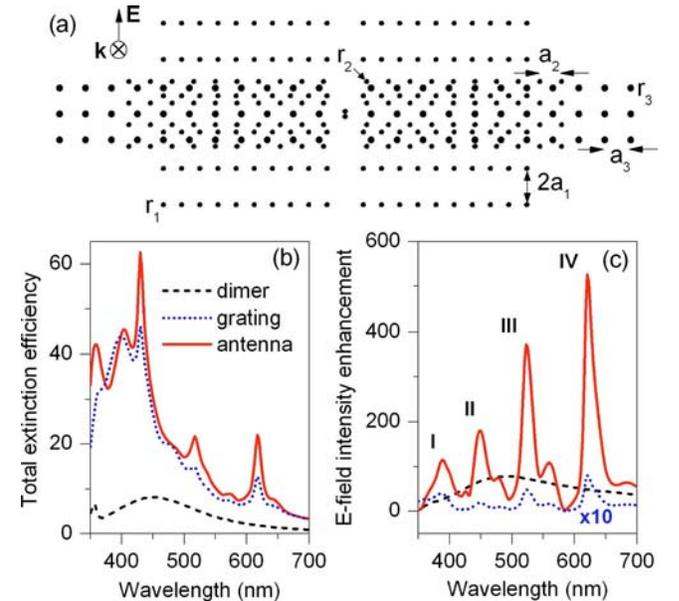
Fig. 3. (Color online) Multiple-wavelength photonic-plasmonic antenna. (a) Schematic of the multiple-wavelength antenna ( $r_1=50$  nm,  $a_1=420$  nm,  $r_2=55$  nm,  $a_2=500$  nm,  $r_3=70$  nm, and  $a_3=600$  nm). Total extinction efficiency (b) and focal point intensity enhancement (c) in the dimer (dashed), multiple-periodic grating without a dimer (dotted) and grating-assisted antenna (solid) as a function of wavelength.
