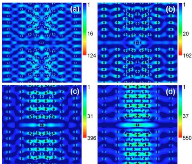
Fig. 4. (Color online) Near-field intensity distributions (log scale) in the multiple-wavelength antenna at the wavelengths ( $\lambda_1=388$  nm,  $\lambda_2=449$  nm,  $\lambda_3=523$  nm, and  $\lambda_4=621$  nm) corresponding to the four peaks in Fig. 3(c). At each wavelength, a high-intensity hot spot is created in the dimer gap.
