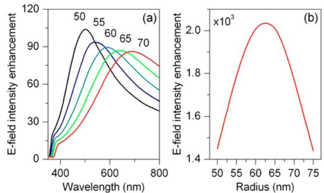
Fig. 5. (Color online) Optimization of the dimer-grating coupling efficiency. (a) Focal point intensity in a bare dimer (gap 15 nm) as a function of wavelength and the radii of the nanoparticles (labeled in the units of nm). (b) Scaling of the focal point intensity in the optimized ( $r=95$  nm) 20-period six-arm single-wavelength antenna [same as in Fig. 2(d)] with the radii of the particles in the dimer.
