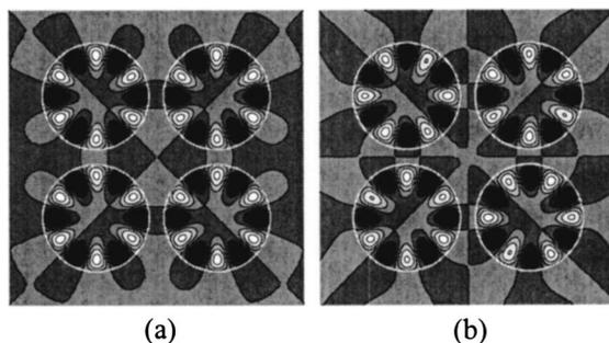
Fig. 4. Magnetic near-field portraits of the (a) OE and (b) OO modes in the square molecule with  $d = 1.45 \mu\text{m}$ .
