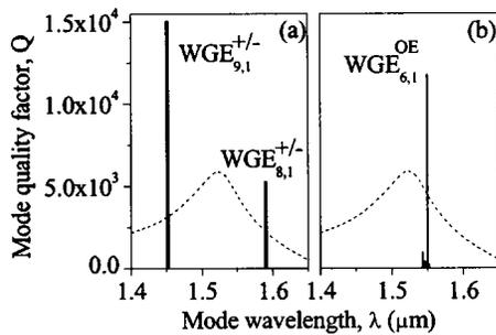
Fig. 5. Spectral lines with respective  $Q$  factors for the WG modes in (a)  $2.3\ \mu\text{m}$  diameter single microdisk and (b) optimally tuned ( $d=1.6125\ \mu\text{m}$ ) square photonic molecule composed of  $1.8\ \mu\text{m}$  diameter microdisks. The dotted curve is an approximation (a.u.) of the spontaneous emission spectrum in GaInAsP–InP quantum well microdisk lasers (Ref. 12).
