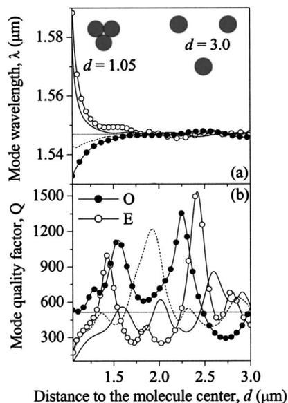
Fig. 1. Shift and splitting of wavelengths (a) and change of  $Q$  factors (b) of the  $\text{WGE}_{6,1}$  modes in a triangular photonic molecule as a function of the cavities' distances to the molecule's center. Corresponding single-cavity characteristics are plotted for comparison (straight line).
