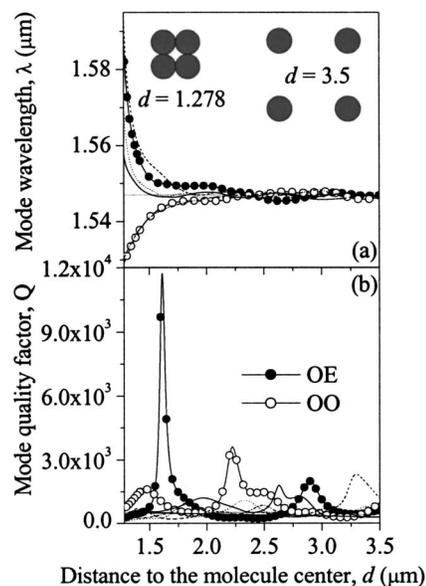
Fig. 3. Shift and splitting of wavelengths (a) and change of  $Q$  factors (b) of the  $\text{WGE}_{6,1}$  modes in a square photonic molecule as a function of cavities' distances to the molecule center.
