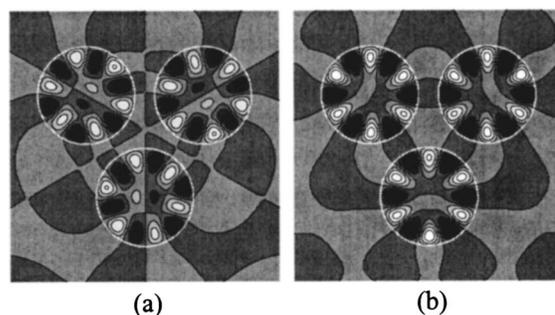
Fig. 2. Magnetic near-field portraits of the (a) O and (b) E modes in the triangular molecule with  $d = 1.25 \mu\text{m}$ .
