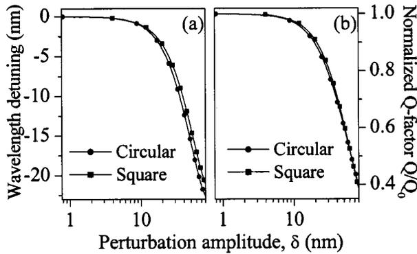
Fig. 6. (a) Resonant wavelength detuning and (b)  $Q$ -factor degradation of the  $WG_{5,1}$  mode of the circular microdisk and WG-like mode of the square microcavity as a function of the depth of the mismatched contour perturbation with the period  $\Lambda = 0.033$  ( $\nu = 30$ ).
