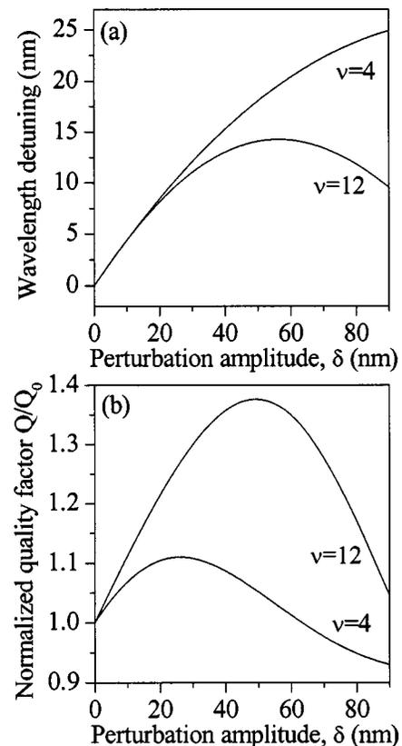
Fig. 4. (a) Resonant wavelength shift and (b) normalized  $Q$ -factor change versus the perturbation amplitude  $\delta$  for the two types of the favorably matched deformation of the square microcavity ( $\nu = 4$  and  $\nu = 12$ ).
