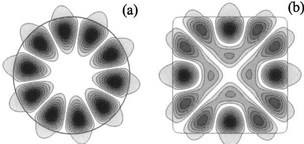
Fig. 1. Field intensity distributions for (a) the  $\text{WG}_{5,1}$  mode of the circular microcavity ( $\lambda = 1.572 \mu\text{m}$ ) and (b) the WG-like mode of the square microcavity ( $\lambda = 1.503 \mu\text{m}$ ). The cavities have a diameter (side length) of  $1.6 \mu\text{m}$  and permittivity  $\epsilon = 6.9169 + i10^{-4}$ .
