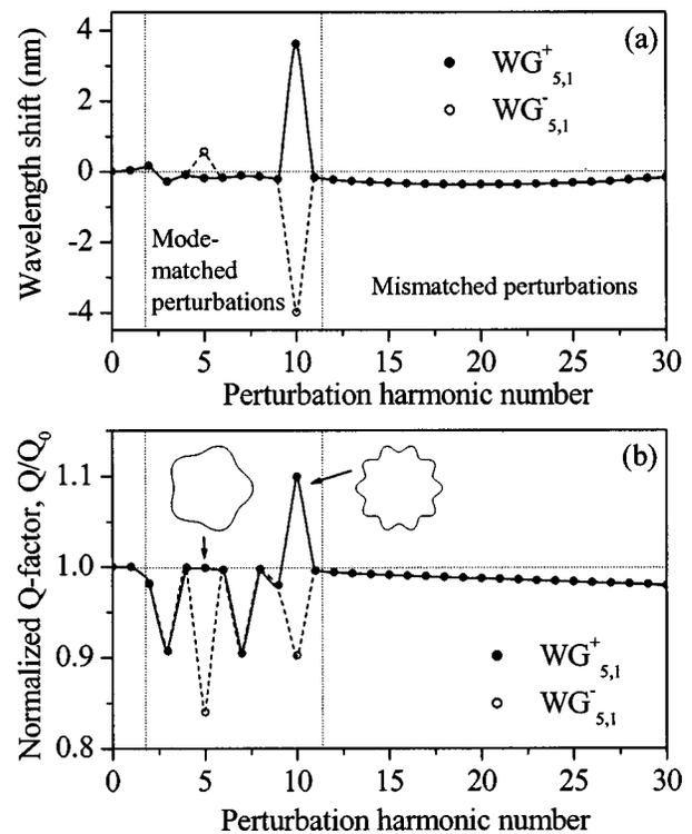
Fig. 2. (a) Circular microcavity resonant wavelength detuning and (b) normalized loss-limited  $Q$  factor as a function of the contour perturbation harmonic number  $\nu$ . Radial depth of the perturbation is  $\delta = 8 \text{ nm}$ . Regions of the mode-matched perturbations and mismatched surface roughness can be observed. The inset shows two favorably mode-matched contour deformations ( $\nu = 5$  and  $\nu = 10$ ).
