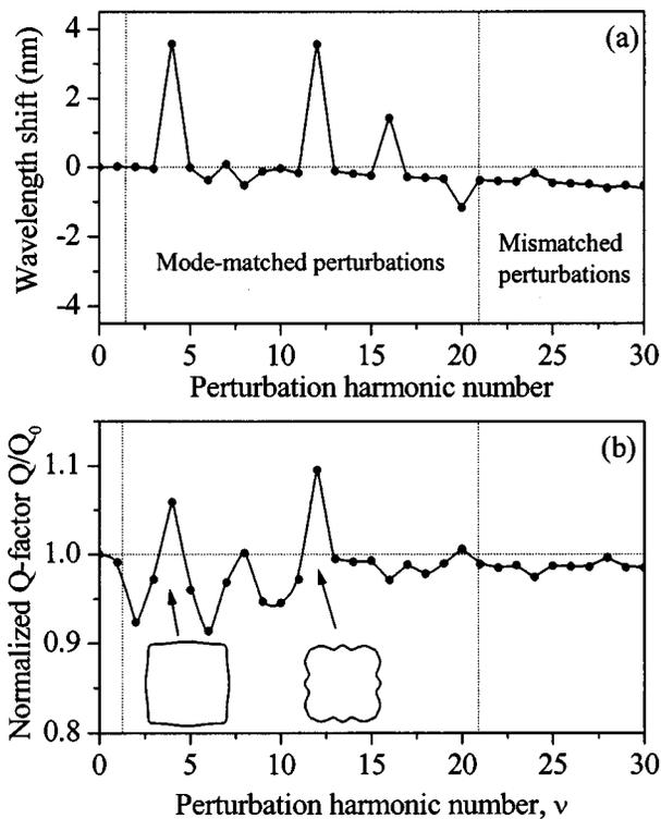
Fig. 3. (a) Square microcavity resonant wavelength detuning and (b) normalized loss-limited  $Q$  factor as a function of the contour perturbation harmonic number  $\nu$ . Radial depth of the perturbation is  $\delta = 8$  nm. Two types of the favorably mode-matched deformation ( $\nu = 4$  and  $\nu = 12$ ) are shown in the inset.
