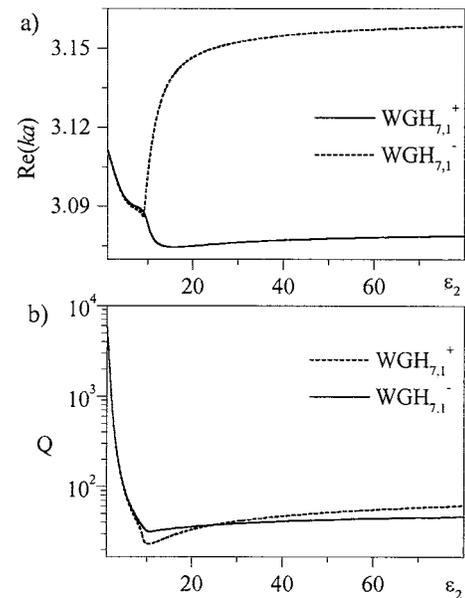
Fig. 6. (a) WGM resonance frequencies and (b)  $Q$  factors of DR over the dielectric boundary versus the permittivity of the lower half-space.  $w/a = 0.001$ ,  $\epsilon_b = 10 + 0.001i$ ,  $\epsilon_1 = 1$ .
