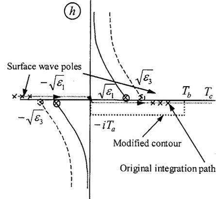
Fig. 2. Complex  $h$  plane and the contour of integration chosen for numerical evaluation of spectral integrals.
