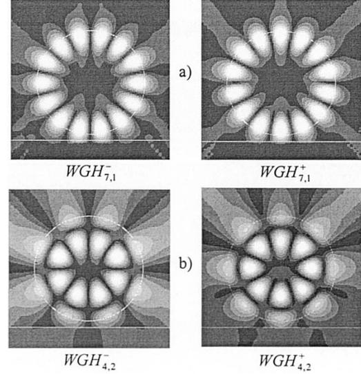
Fig. 3. Fields patterns of (a)  $WGH_{7,1}^{\pm}$  and (b)  $WGH_{4,2}^{\pm}$ . Both are resonances of the DR located over the grounded dielectric slab waveguide with parameters  $d/a = 1$ ,  $\varepsilon_b = 10 + 0.001i$ , and  $\varepsilon_2 = 4.8$ .
