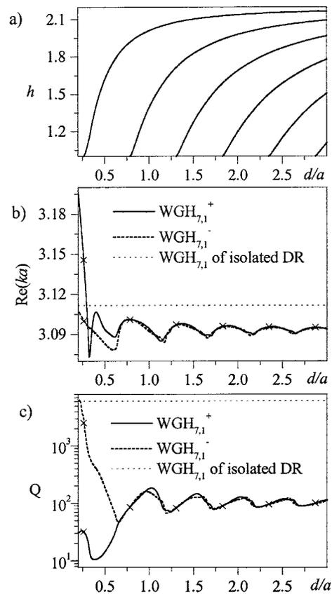
Fig. 5. Normalized propagation constants of the (a) grounded dielectric-slab eigenmodes, (b) WGM natural frequencies, and (c)  $Q$  factors of DR versus the slab thickness  $w/a = 0.01$ ,  $\epsilon_b = 10 + 0.001i$ ,  $\epsilon_2 = 4.8$ .
