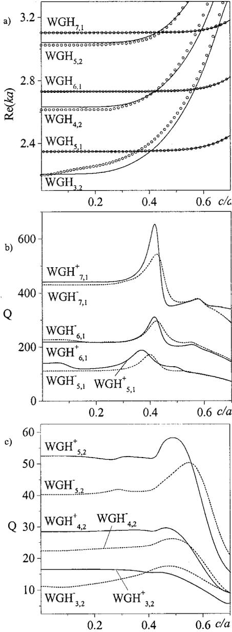
Fig. 7. Resonance frequencies and  $Q$  factors of WGMs of a ring DR located over a grounded dielectric slab versus the inner radius of the resonator.  $w/a = 0.01$ ,  $d/a = 1$ ,  $\varepsilon_b = 10 + 0.001i$ ,  $\varepsilon_2 = 4.8$ . In (a), the solid lines are for the (+) oscillations, and the circles are for the (-) ones.
