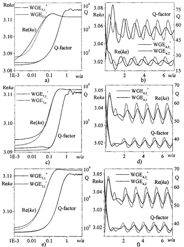
Fig. 4. Shift of the WGM resonance frequencies of a circular-cylindrical DR ( $\epsilon_b = 10 + 0.001i$ ) in the free half-space ( $\epsilon_1 = 1$ ) due to the presence of (a), (b) dielectric-dielectric interface ( $\epsilon_2 = 9$ ); (c), (d) grounded dielectric-slab waveguide ( $d/a = 1$ ,  $\epsilon_2 = 4.8$ ); (e), (f) asymmetrical dielectric waveguide ( $d/a = 1$ ,  $\epsilon_2 = 6$ ,  $\epsilon_3 = 4$ ).
