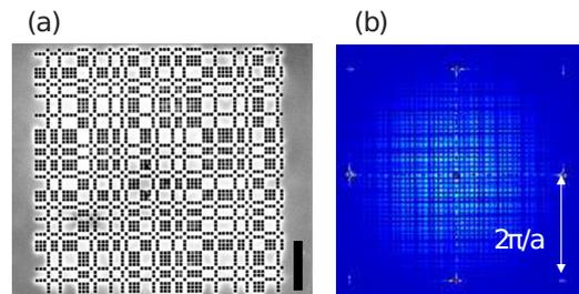
FIG. 1. (Color online) (a) SEM image of a 2D array of air holes arranged in the Rudin-Shapiro sequence in a free-standing GaAs membrane. The black vertical bar is  $5 \mu\text{m}$ . (b) Reciprocal space representation of the structure obtained by Fourier transform of the SEM image. The nine spots around the boundary correspond to the reciprocal vector of square lattice with the lattice constant  $a = 380$  nm.
