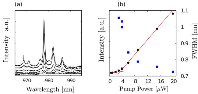
FIG. 2. (Color online) (a) Emission spectra taken at the incident pump power  $P=3, 4.1, 6, 9, 15, 20 \mu\text{W}$ . (b) Measured intensity (black circle) and spectral width (blue square) of one emission peak at wavelength  $\lambda=978 \text{ nm}$  vs  $P$  showing the onset of lasing at  $\sim 3 \mu\text{W}$ . The solid lines are linear fitting of peak intensity below and above the threshold pump power ( $\sim 3 \mu\text{W}$ ).
