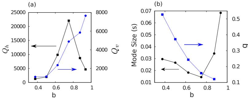
FIG. 4. (Color online) (a) Calculated  $Q_h$  and  $Q_v$  for the highest- $Q$  modes vs  $b$ .  $Q_h$  becomes maximal at  $b=0.75$  while  $Q_v$  increases monotonically with  $b$ . (b) Lateral size  $s$  of the highest- $Q$  mode and percentage  $g$  of the continuous background in the spatial Fourier spectra of the Th-Mo structures as a function of  $b$ .  $s$  is minimal near the optimal value of  $b$  where  $Q_h$  is maximal.  $g$  decreases monotonously as  $b$  increases.
