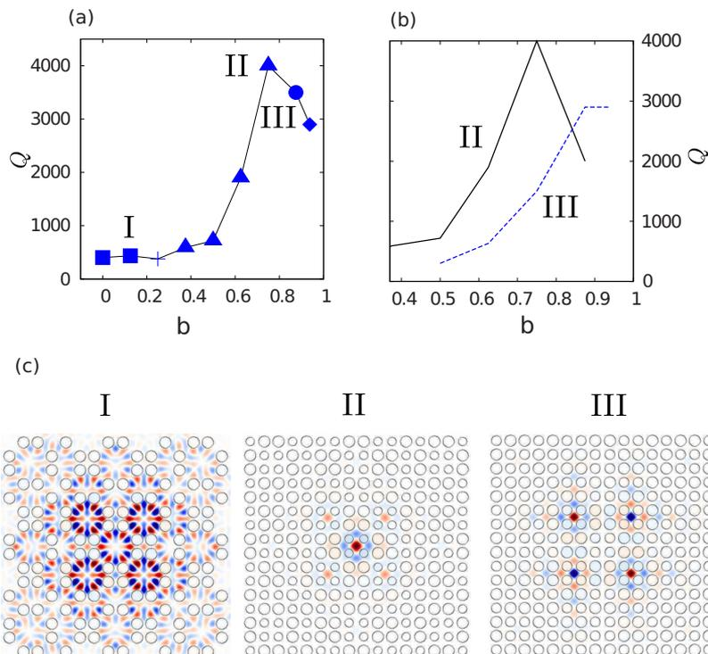
FIG. 3. (Color online) (a) Calculated  $Q$  values of the highest- $Q$  modes for each  $b$ . Different symbols represent different types of modes, e.g., square for type I, triangle for type II, and circle for type III. (b)  $Q$  factor as a function of  $b$  for type II (black curve) and III (blue dashed curve) modes. (c) Spatial distribution of magnetic field for type I, II, and III modes (from left to right). Type II becomes the overall maximal- $Q$  mode at  $b=0.75$ .
